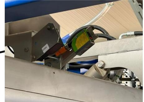
When a Buffalo enters the robot, the **Photoelectric sensors output** switch from:
