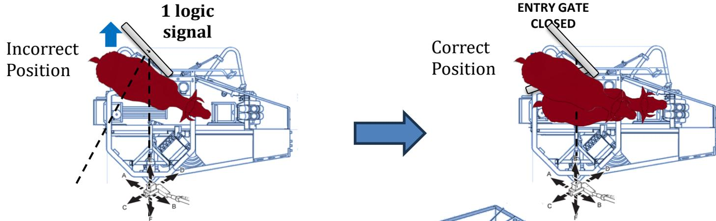
Then, after a few seconds the closing of the entry gate, the robotic arm moves towards Buffalo udder, to attach the milking cluster and began milking routine.
