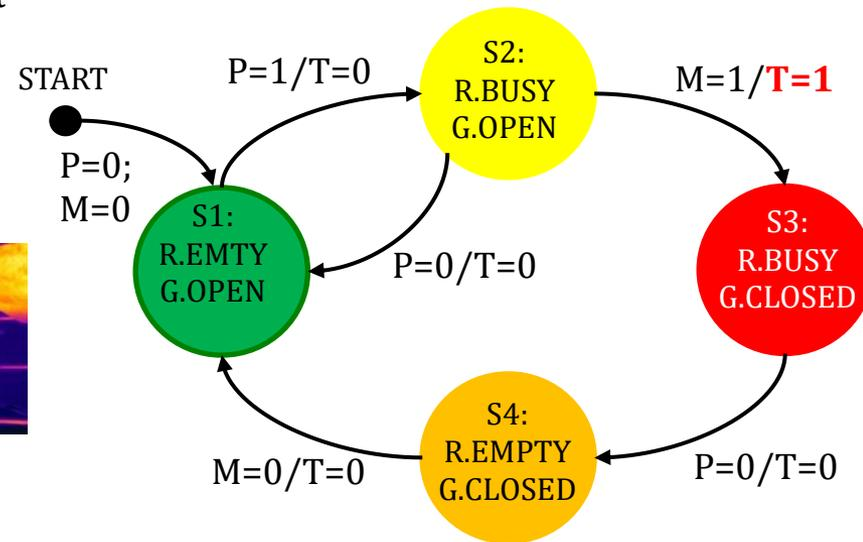
The Firmware running on Microcontroller is based on a Finite State Machine (FSM) that takes two inputs, Photoelectric Sensor (P) and Magnetic Contact Sensors (M) and generate a single output, i.e., the **suitable trigger signal (T)** for the Infrared Camera, which captures a thermal snapshot of the udder.
