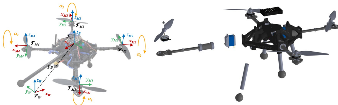
Figure 2: Prototype of the omnidirectional quadrotor with model description (left) and exploded version with components (right).
