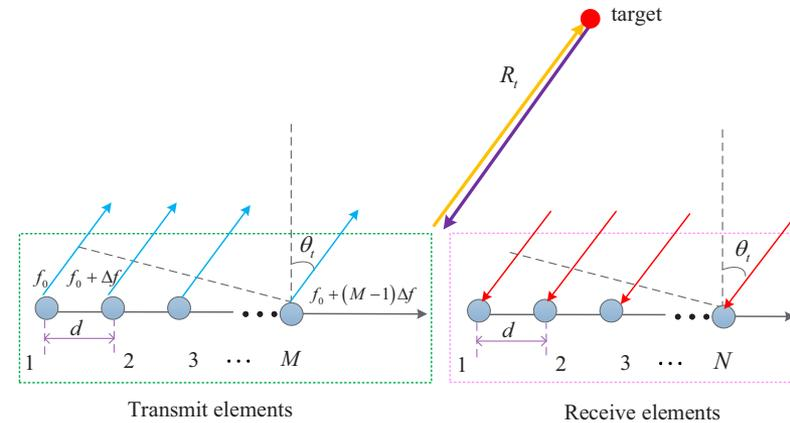
Signal transmission and reception in FDA-MIMO radar.
