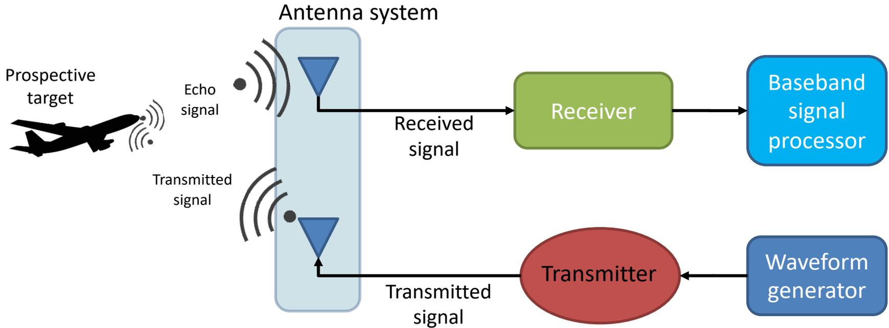
**Block diagram of a conventional radar system**
