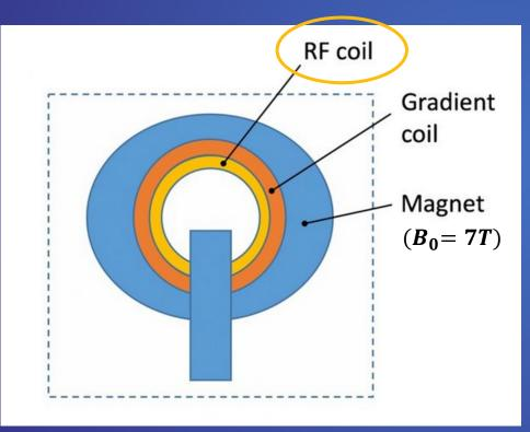
Signal to noise ratio proportional to the static magnetic field
