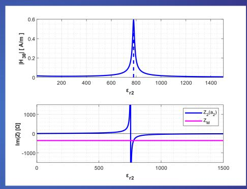
HPM relative Permittivity equal to 780 can amplify selectively the fundamental mode!
